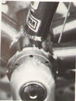
Ovalized tubing on Fisher Excaltur
