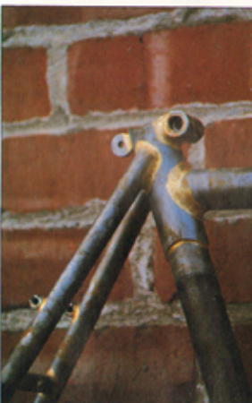
Fillet brazing of an unpainted Salsa frame.
