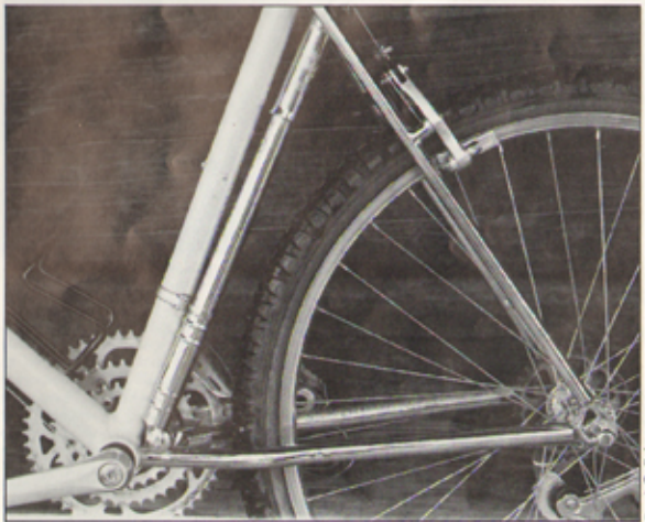
Mantis composite/aluminum main triangle with steel rear triangle
