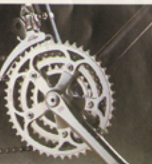
SunTour derailers, Specialized crankset and sealed bottom bracket.
