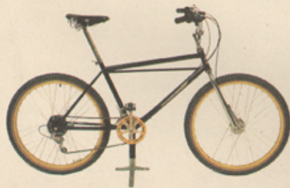
1979 Lanesville Knight Pro cruiser 5-speed owned by Mert Lanesville. Sturmev-Archer Drum brakes, Tomaselli brake levers, Mert Lanesville custom stem, motorcycle handlebars, SunTour thumbshifter and rear derailleur.
