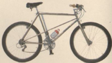
1977 Breeze owned by Charles Kelly. Second Breeze built, equipped with Phil Wood hubs, Magna handlebars and brake levers, SunTour thumbshifters and derailleurs, Weinman cantilever brakes, Campagnolo seatpost with custom modification to accept Brooks B-72 saddle, TA cranks, Cook Brothers fork custom modified by Joe Breeze.
