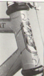
The Trench Goat even has the same fillet brazing applied to the back of the head tube reinforcement rings, just like the American built Goats.
