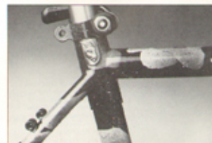
The reinforced seat collar, not only offers a stronger seatpost, but lets you attach your Hite-Rite™ without interfering with your quick release seatpost binder bolt.
