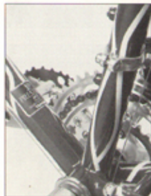
Note the surface mounted water bottle bosses. This reduces the number of holes drilled into the frame. Wiggle Wipe paint finish.
